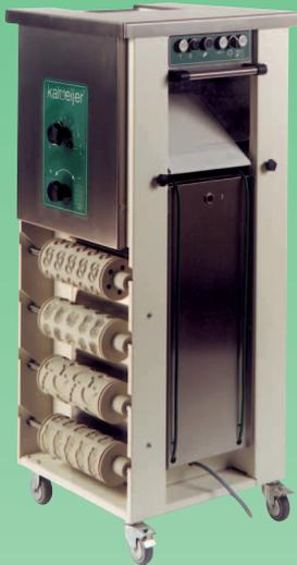
Saving of space: 550 x 570 mm, because the baking tray tables and the feed hopper for the dough transport are collapsible.
