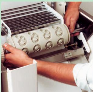
Changing the figure roller without using any tools, that is also the case for cleaning the feeding roller.
