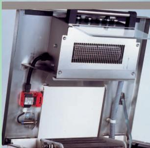
Heating system has been mounted in the cover.
