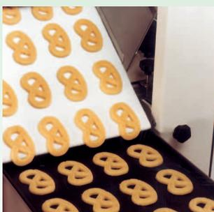
The dough figures drop on to the baking tray in straight lines.
